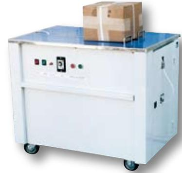
This fully portable strapping machine dispenses, tightens, and seals economical polypropylene strapping around packages or bundles greater than 3". Unit automatically tensions strap and joins the ends with a secure heat weld. The motor automatically switches off when not in use. As the strap is inserted, the motor automatically restarts. Wall plug is standard 115V single phase 15 amp.
