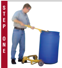
STEP ONE Align unit in front of drum, remove handle, grip drum with the handle
