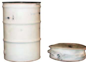
Crushes a drum to approximately 6" high
